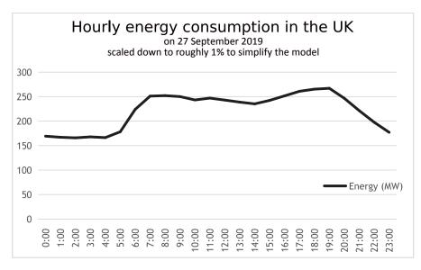
Fig. 3. Usage data for the UK, scaled down to about 1%, in MW, across 24 hours on Friday 27 September 2019 – data obtained from *Balancing Mechanism Reporting Service* (BMRS) [6]
